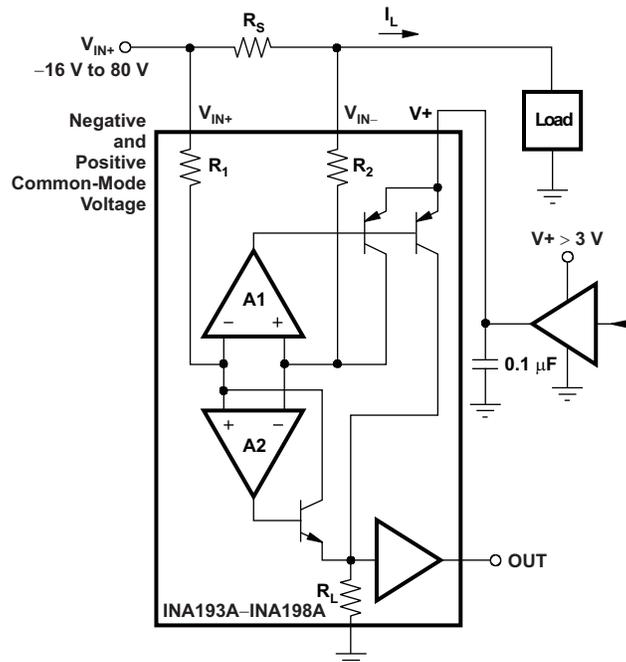
**Figure 4. INA193A–INA198A Example Shutdown Circuit**
