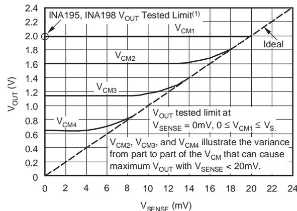
NOTE: (1) INA193, INA196  $V_{OUT}$  Tested Limit = 0.4V.
